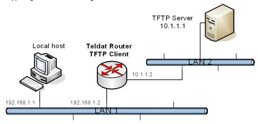
We want to remotely download a code release (newatlas.bin) as well as a new configuration file (newatlas.cfg) for the router. Both files are stored in a TFTP server, accessible through the device.
